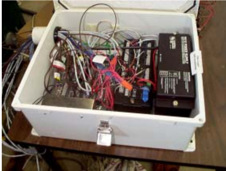
Figure 8. Data logger to collect flow and temperature data
