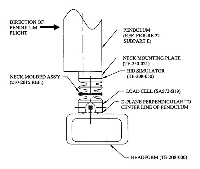
NOTE: MOUNT NECK AT LEADING EDGE OF PENDULUM TO AVOID INTERFERENCE WITH HEADFORM MOTION. PENDULUM SHOWN IN VERTICAL ORIENTATION. FIGURE 9D
