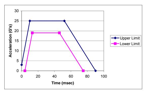
**CONFIGURATION I ACCELERATION FUNCTION CURVE** ACCELERATION FUNCTION FOR  $\Delta V = 48 \text{ km/h} (30 \text{ mph})$
