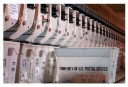
New Postal Service automation equipment is capable of processing flat-size mail at a rate of over 17.000 pieces per hour! This high speed processing not only helps to hold down postal operating costs and, consequently, postage rates, it also enables consistency in on-time mail delivery. High readability of barcode and address information is a critical component of automation success.
