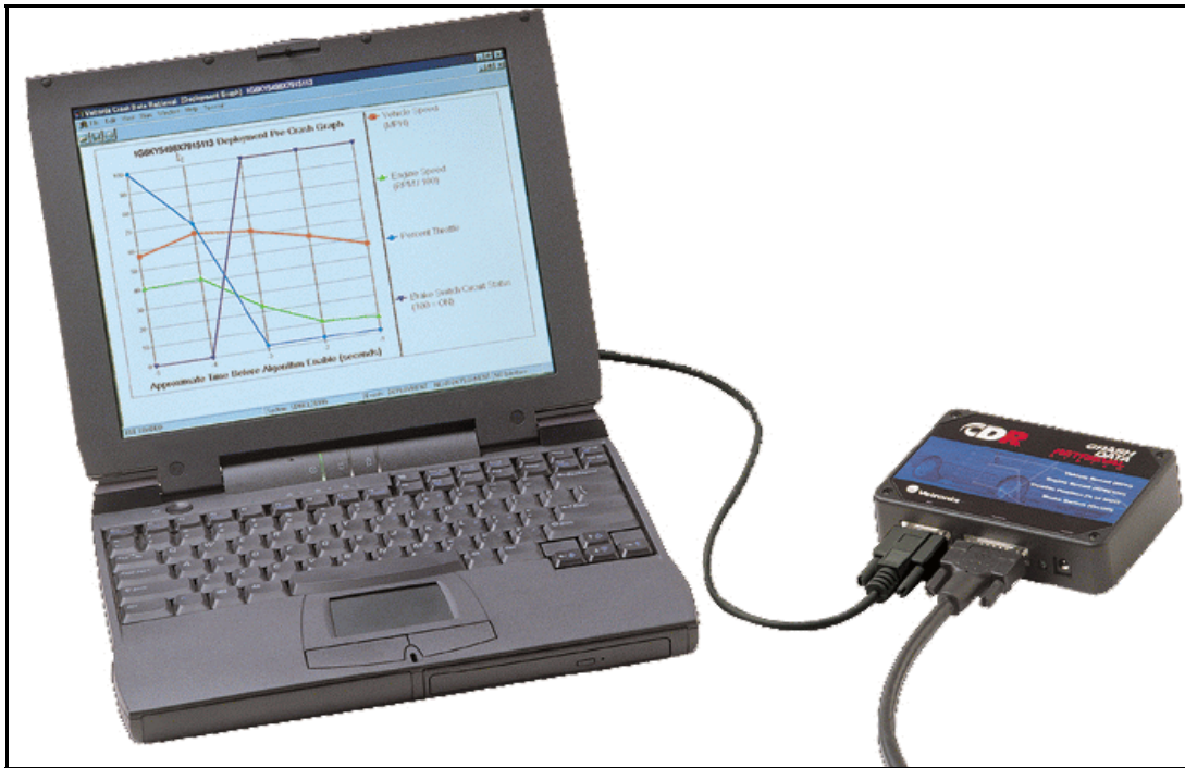
Figure 4. Vetronix EDR Data Retrieval System.
