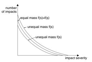
Figure 1. Impact severity (delta-V) for cars in matching crashes for equal mass:  $f_1(s) = f_2(s)$  and unequal mass:  $f_1(s) \neq f_2(s)$  where car 1 is of less mass than car 2.
