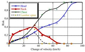
Figure 7. Injury risk for head, chest, neck and lower spine injuries versus change of velocity from crash pulse recorder data.
