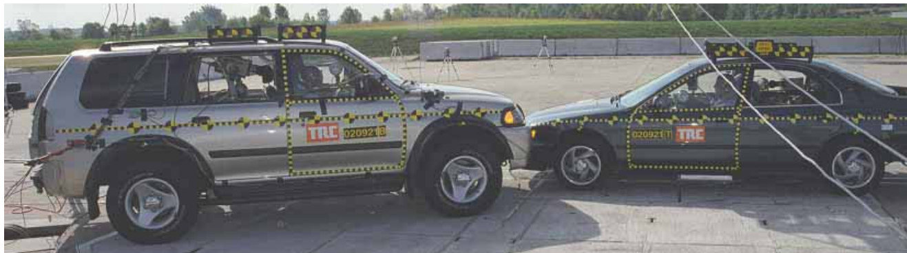
1999 Montero Sport (IIHS rated “poor”) (4646 lbs, Width=1705 mm)
