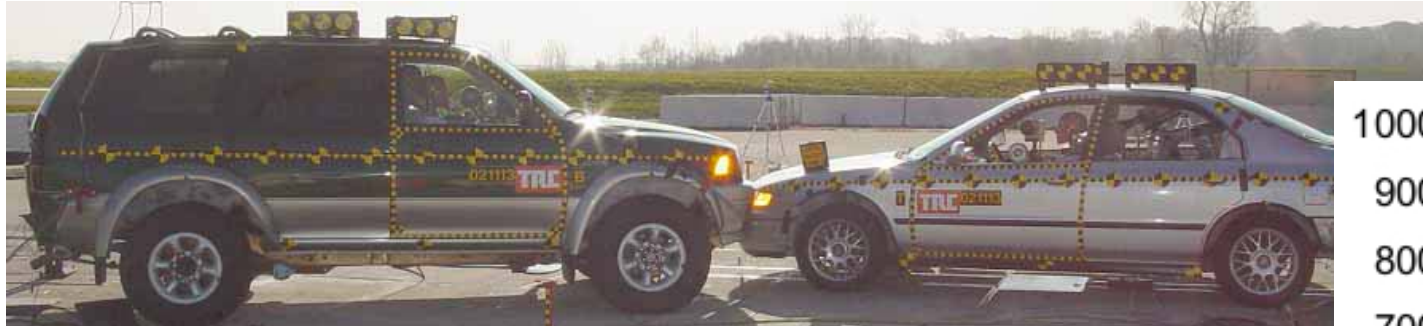
1999 Montero Sport (IIHS rated “poor”) (4646 lbs, Width=1705 mm)
