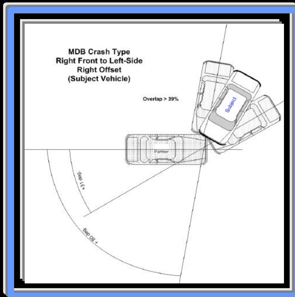
MDB type crash with a right oblique right offset configuration
