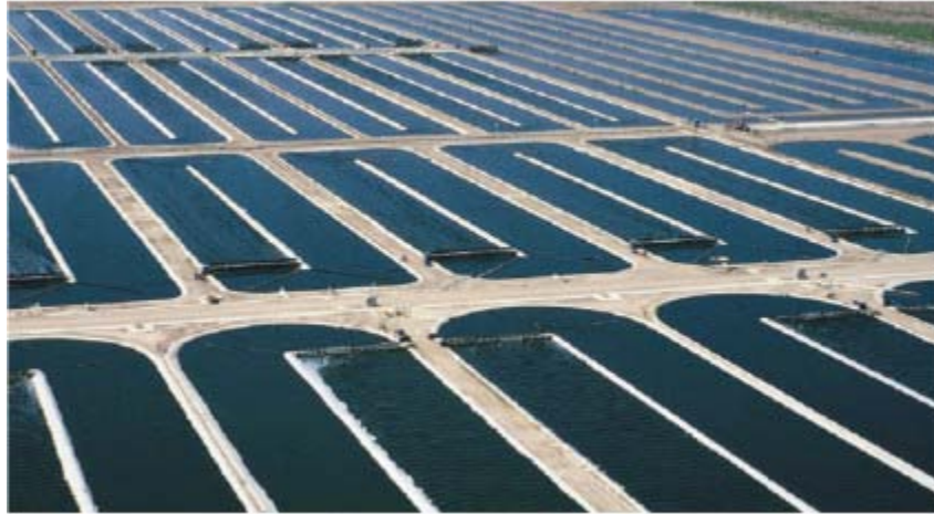
Figure C-13. Example of an Open Pond Raceway System
