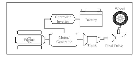
Figure 3-3 Schematic of Honda IMA System [Husted, 2003]
