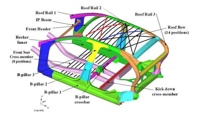
Figure 3-4: Example of CAE optimization of the design and position of the roof rails and front seat cross-member for the "Future Generation Passenger Compartment." The thin lines represent relative positions for roof bows and front cross-members considered during iterations of the CAE analysis of the vehicle structure. The different colors given to the structural components represent differences in sectional material thickness within this particular CAE modeling run.
