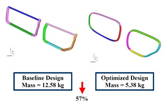
Figure 3-6: Example of CAE optimization of a door-beam design for the "Future Generation Passenger Compartment" that reduces component mass by 57% and reduces part count and assemby. 53
