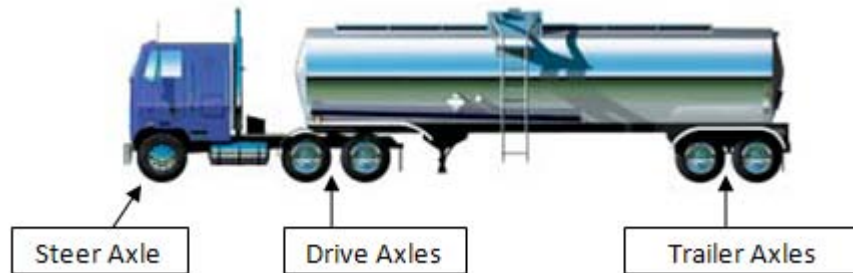
Figure 1-21 Class 8 Standard "18 Wheeler" Axle Identification
