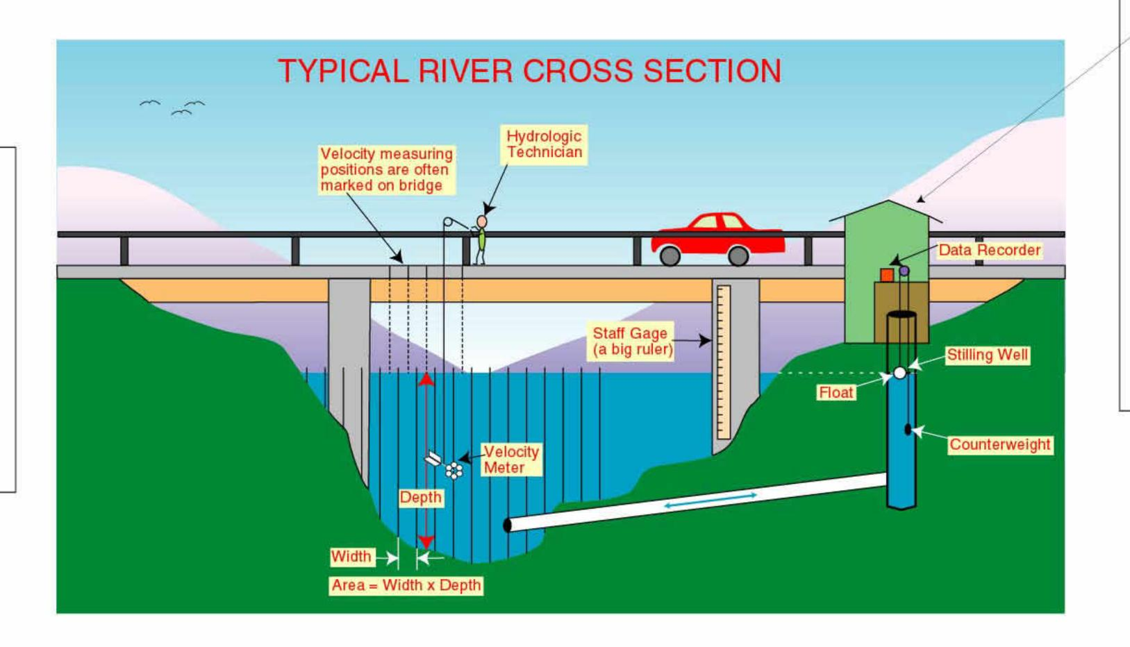
In the gage house there is equipment which records gage height (level of water surface) every 15 minutes and stores this data. Other data such as water temperature and pH can also be recorded. For some sites this data is transmitted to our office via satellite so that we can watch water level changes as they are happening.
