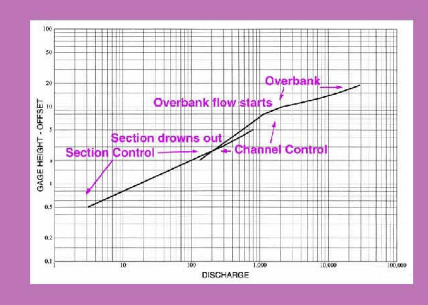
A rating curve is a graphical representation of the relationship between stage (water level) and discharge for a given stream or river. The rating curve is developed from discharge measurements collected over a period of time and over a range of stages (from low flow to flood stage). Each point on the graph represents one discharge measurement. This rating curve can be used to estimate discharge at a given gage height.
