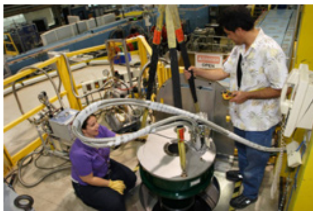
NCNR's Sarah Parks and Juscelino Leão lower the 10 T magnet into the DCS sample well.
