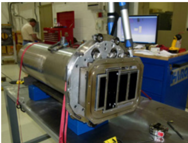
FIGURE 5: The in-pile plug containing the metal-substrate supermirror guides comprising the first section of the new guide network.
