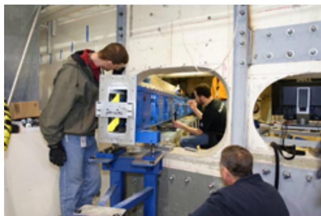
FIGURE 7: Danny Ogg and Mike Rinehart work with Dan Adler (center) in aligning the vacuum-jacketed NG-D guide inside the D-wing.
