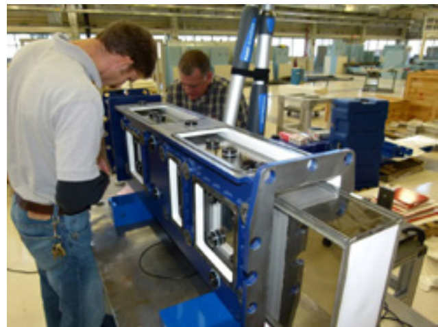
FIGURE 4: Doug Ogg (left) and Mike Rinehart use a measuring arm to characterize an element of guide NG-C.
