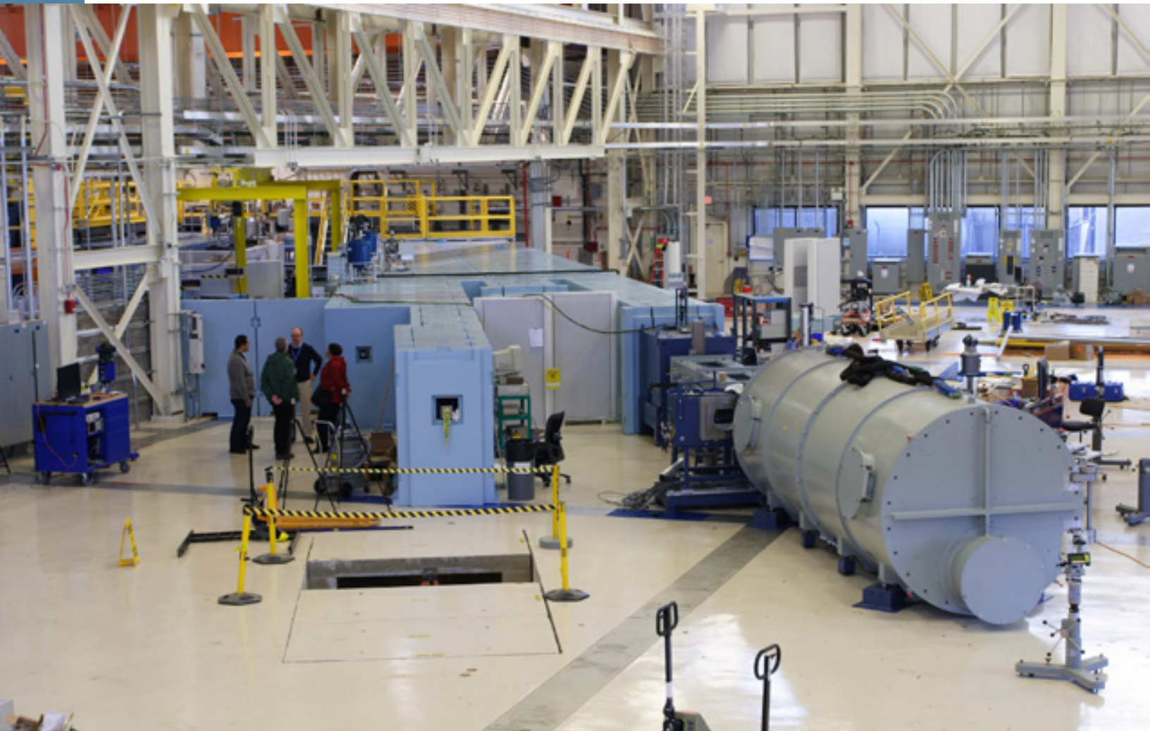
A view of new guides emerging into the guide hall in a Nov. 6, 2012 photo. The group of people is standing by NG-D, emerging through the square hole just to their right. Behind them are shields blocking the view of the newly installed PBR and MAGIk instruments, taking beams off the side of NG-D. The guide visible just behind the striped safety marker is NG-C, and to its right, emerging from NG-B lower , is the tank of the 10 m SANS instrument being installed. NG-B upper is behind the two grey shields to the left of the tank. Not visible is NG-A, to the right of the 10 m SANS, still under development.
