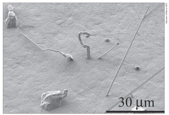
Tin solders without lead are prone to spontaneously sprout whiskers, which can short circuit sensitive electronics. The Material Measurement Laboratory provides measurements and data necessary for industry to change their production methods to prevent the formation of tin whiskers.
