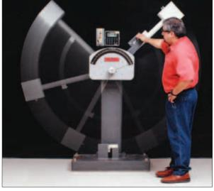
The Charpy impact test uses a swinging pendulum to assess the resistance of a material to fracture.
