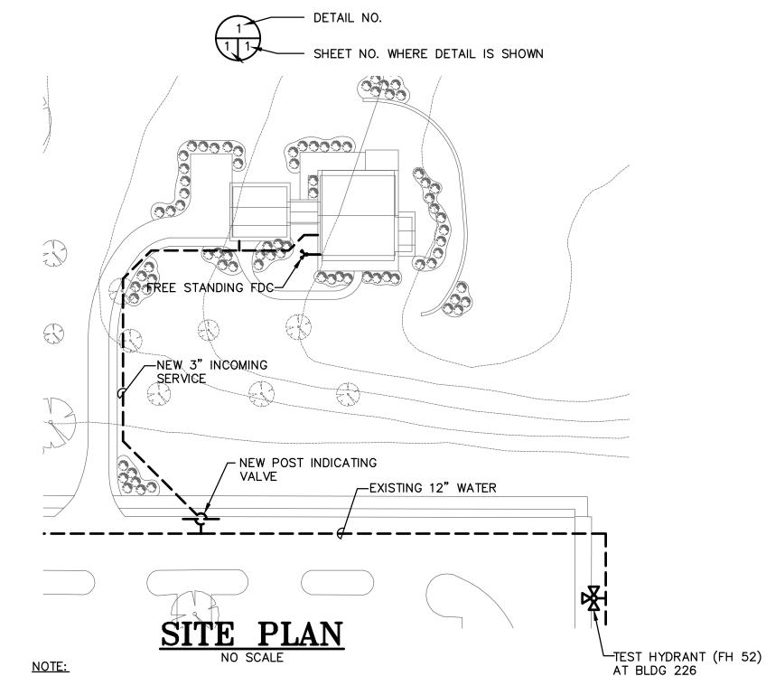
1. ALL PIPING AND HYDRANT LOCATIONS DEPICTED ON THIS PLAN ARE SHOWN FOR THE PURPOSES OF HYDRAULIC CALCULATIONS AND FIRE DEPARTMENT CONNECTION POSITION. THIS SITE PLAN IS NOT INTENDED FOR INSTALLATION OF PIPING AND/OR
