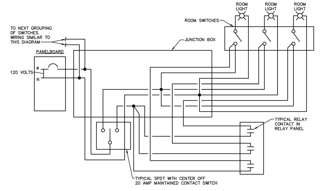
TYPICAL FUTURE WIRING DIAGRAM FOR ROOM SWITCHES E-102, E-104 E-502
