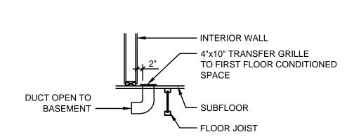
BASEMENT TRANSFER GRILLE DETAIL SCALE:  $\frac{1}{2}$ " = 1'-0"
