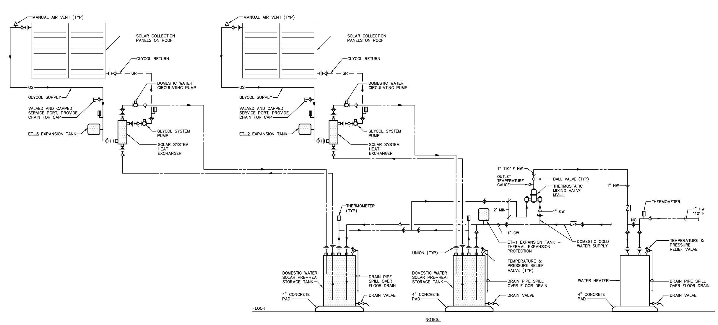
CONTRACTOR TO FOLLOW THE MIXING VALVE MANUFACTURERS RECOMMENDED PIPING FOR COLD, HOT AND RECIRCULATING CONNECTIONS.
