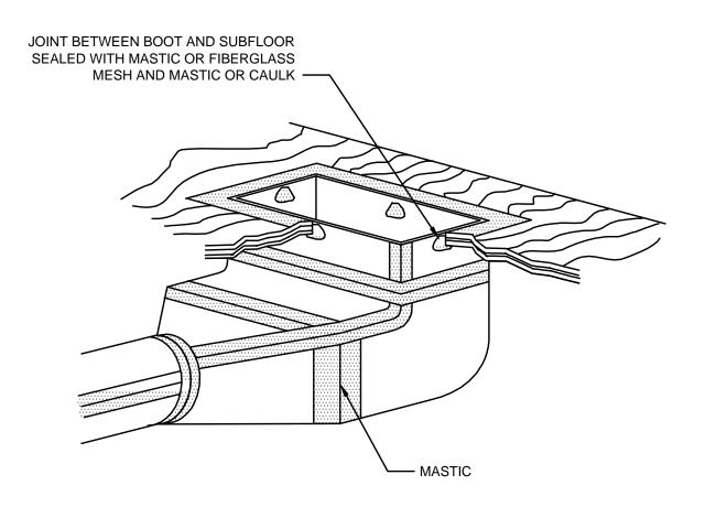
FLOOR BOOT AIR SEALING DETAIL
