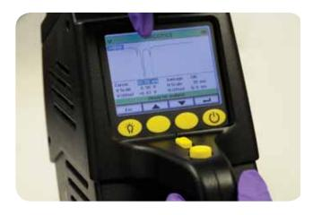
Use of the portable ion mobility spectrometer to screen for active pharmaceutical ingredients in dietary supplements.
