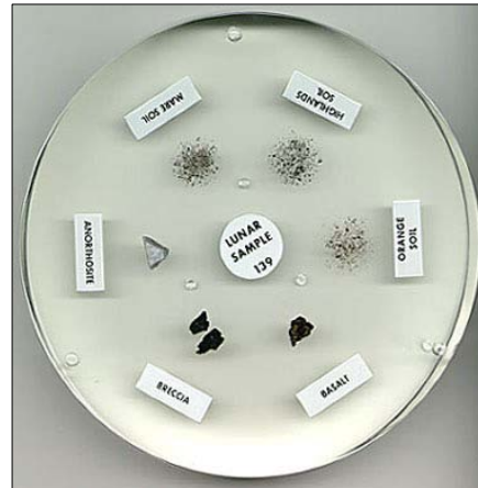
Figure 2. Example of a lunar sample disk. The six-inch diameter disk contains three soil and three rock materials encapsulated in clear acrylic.
