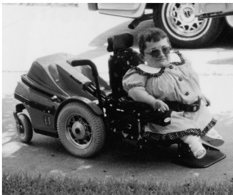
An adult with OI using a power wheelchair with a seat elevator, which allows her to reach things on the floor or on high surfaces.
