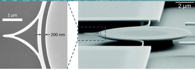
CNST researchers developed a nanomechanical cantilever probe with a high-sensitivity nanophotonic interferometer on a single silicon chip. Replacing the traditional bulky laser detection system with this integrated device allows cantilevers that are orders of magnitude smaller than those used in conventional atomic force microscopy to be built. This innovation creates opportunities for rapid, compact, and low-cost nanoscale metrology for a wide range of applications. (Credit: NIST)
