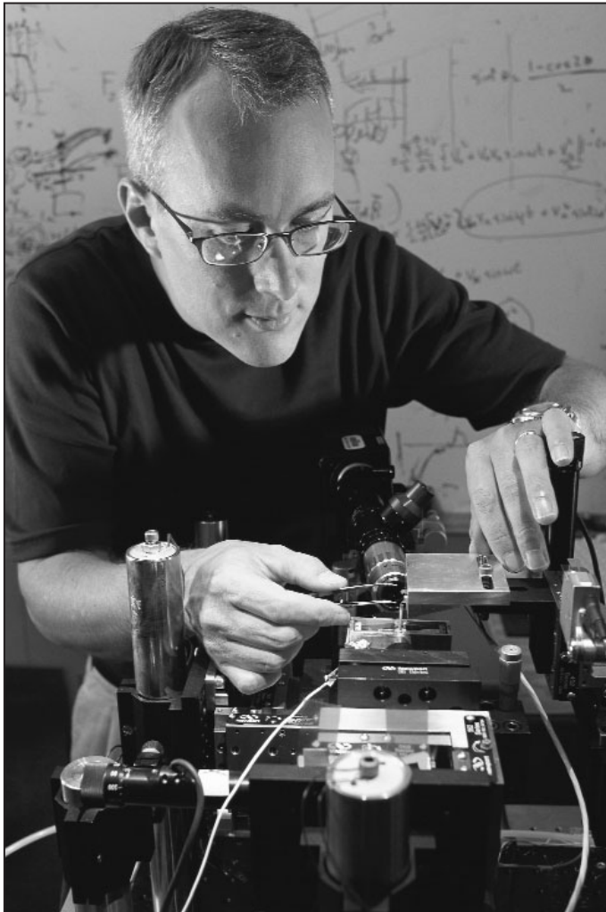
An adjustment is made to the prototype NIST Electrostatic Force Balance designed to measure nanoscale forces.
