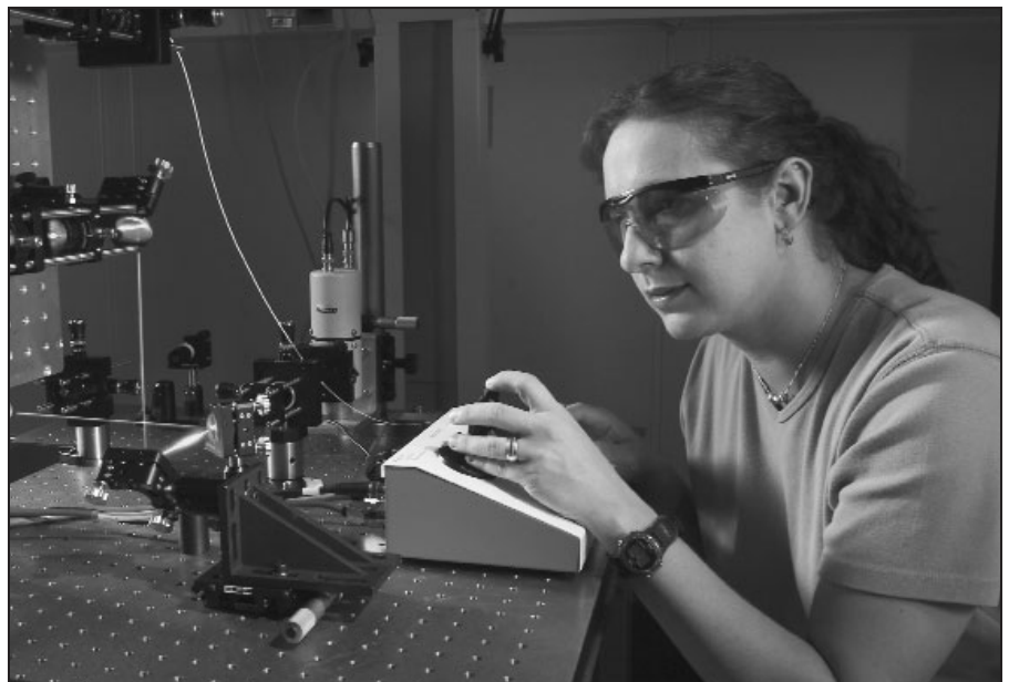
NIST physical scientist positions a tissue-engineering polymer scaffold sample for imaging with a new dual microscope system.
