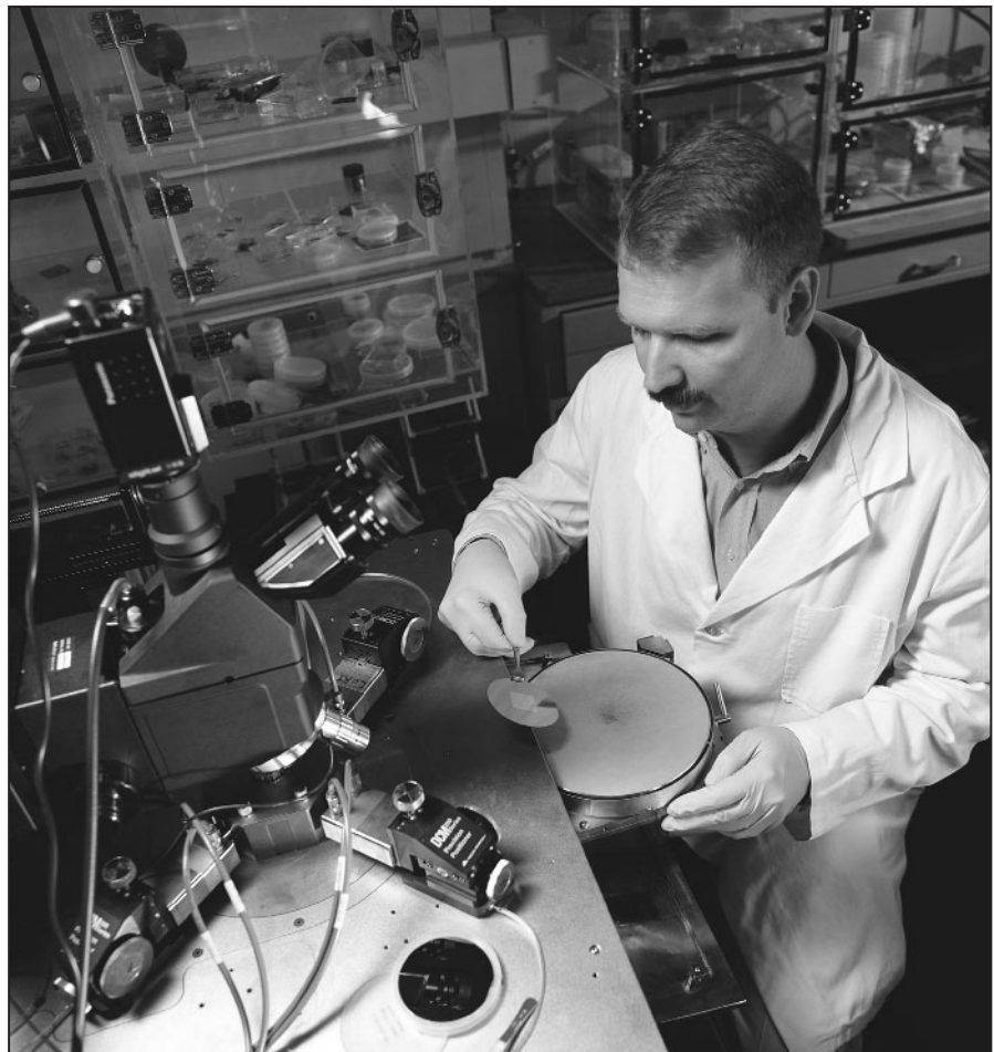
A NIST physicist inserts a wafer into a low-noise electrical probe station as part of a project to develop methods for testing the electrical properties of molecules.
