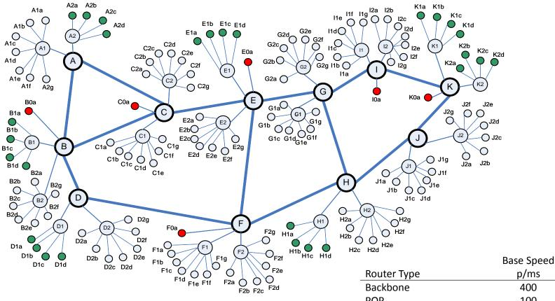
Backbone of Topology based on Internet 2 (including propagation delays & routing paths)
